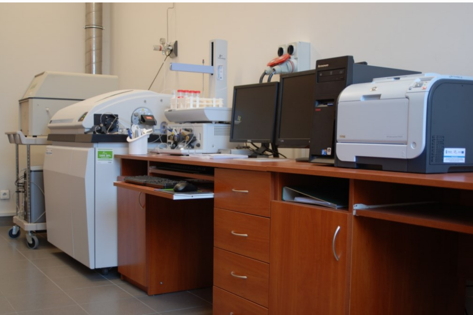
Inductively coupled plasma ionization mass spectrometer with laser ablation module (LA-ICP-MS ELAN DRC II, Perkin Elmer)
